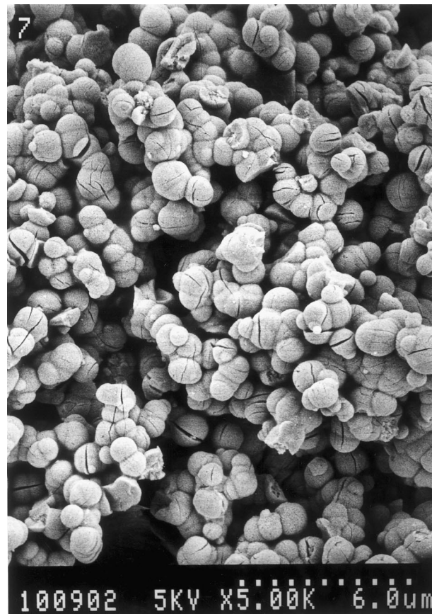
Fig. 6. SEM micrograph of powder prepared with the complexation method.
